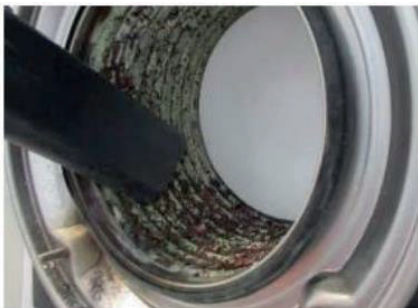
1. Preliminary vacuuming of deposits
